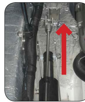
**Remove securing pin,
